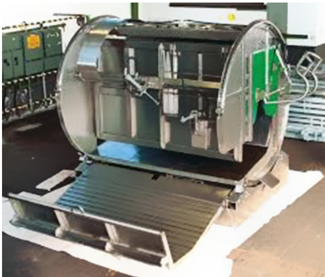
Figure 1.5 Installing the animal before slaughtering in the rotation slaughter box: Weinberg model.
